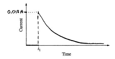
The maximum current occurs just after the switch is closed, when there is no charge on the capacitor.
