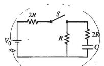
1. The circuit represented above is composed of three resistors with the resistances shown, a battery of voltage  $V_0$ , a capacitor of capacitance C, and a switch S. The switch is closed, and after a long time, the circuit reaches steady-state conditions. Answer the following questions in terms of  $V_0$ , R, C, and fundamental constants, as appropriate.
