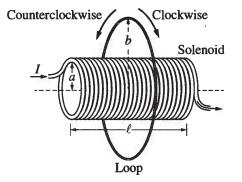
A thin conducting loop of radius b and resistance  $R_L$  is placed concentric with the solenoid, as shown above. The current in the solenoid is decreased from I to zero over time  $\Delta t$ .
