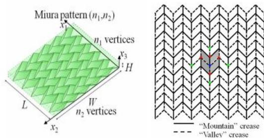
**Figure 1 | Miura-ori.** (left) diagram showing a basic Miura-ori folded tessellation. (right) Crease pattern of the Miura-ori tessellation, showing the folds of a Miura pattern on an unfolded surface [4].
