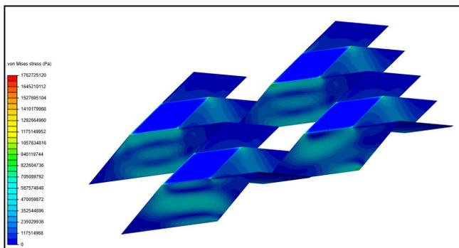
**Figure 3 | Zigzag Base Core Stress Diagram.** The four top faces endured minimal stresses for compression and shear tests, which prompts inquiry into a kirigami-based variation of the pattern that eliminates these faces. Similar recommendations are made for the square twist core.
