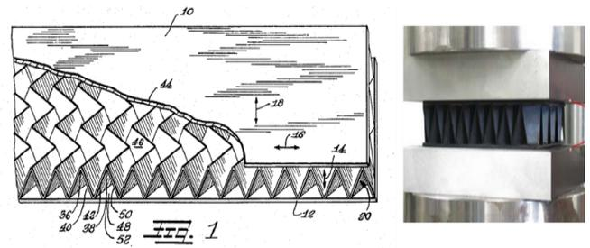
**Figure 2 | Sandwich Panel.** (left) Illustration of a sandwich panel with a Miura-ori folded core [21]. (right) Compression testing of a composite core structure [20].
