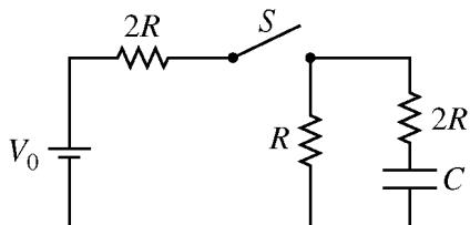
1. The circuit represented above is composed of three resistors with the resistances shown, a battery of voltage  $V_0$ , a capacitor of capacitance  $C$ , and a switch  $S$ . The switch is closed, and after a long time, the circuit reaches steady-state conditions. Answer the following questions in terms of  $V_0$ ,  $R$ ,  $C$ , and fundamental constants, as appropriate.
